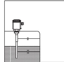
The product is the dielectricum. Due to the higher dielectric constant (DK-value) of the product against air, the capacitance value increases with the height of covering.
